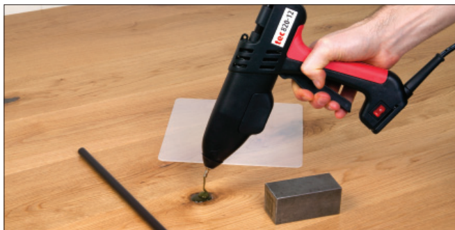
Fast and effective repair of knot defects and other forms of damage
