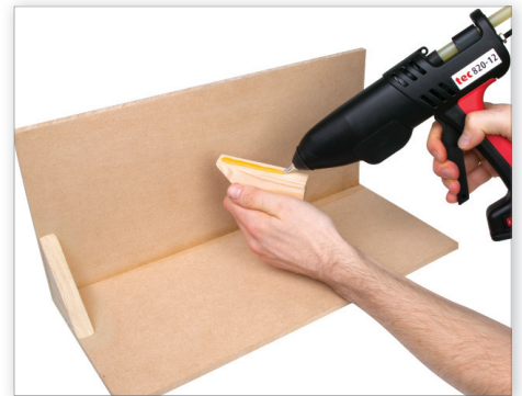
Fasten corner blocks instantly with hot melts
