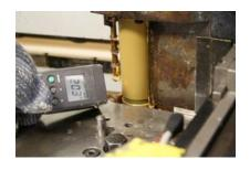
Measure correct temperature on roller and compare it with figure shown on display. Adjust if required.
