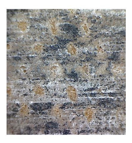
Roller coater set with direct contact to the board giving an uneven coating. (magnified x 40)
